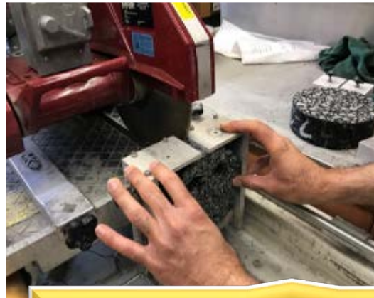
5. Cutting the notch
