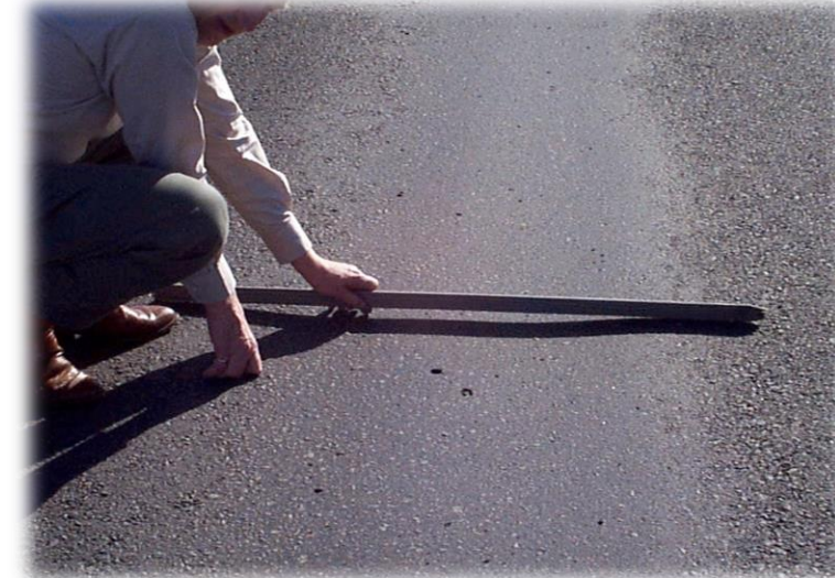
PG 67-22 unmodified, 15mm rut
