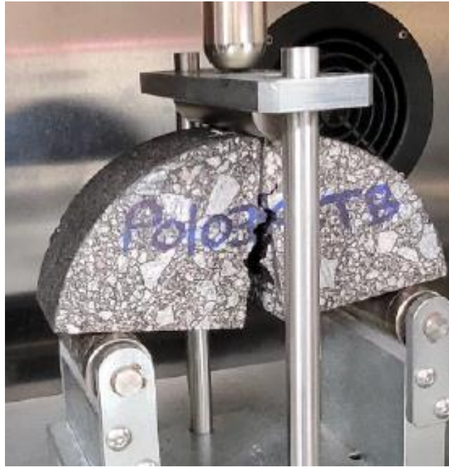
SCB CRACKING RESISTANCE (I-FIT) AASHTO T 393
