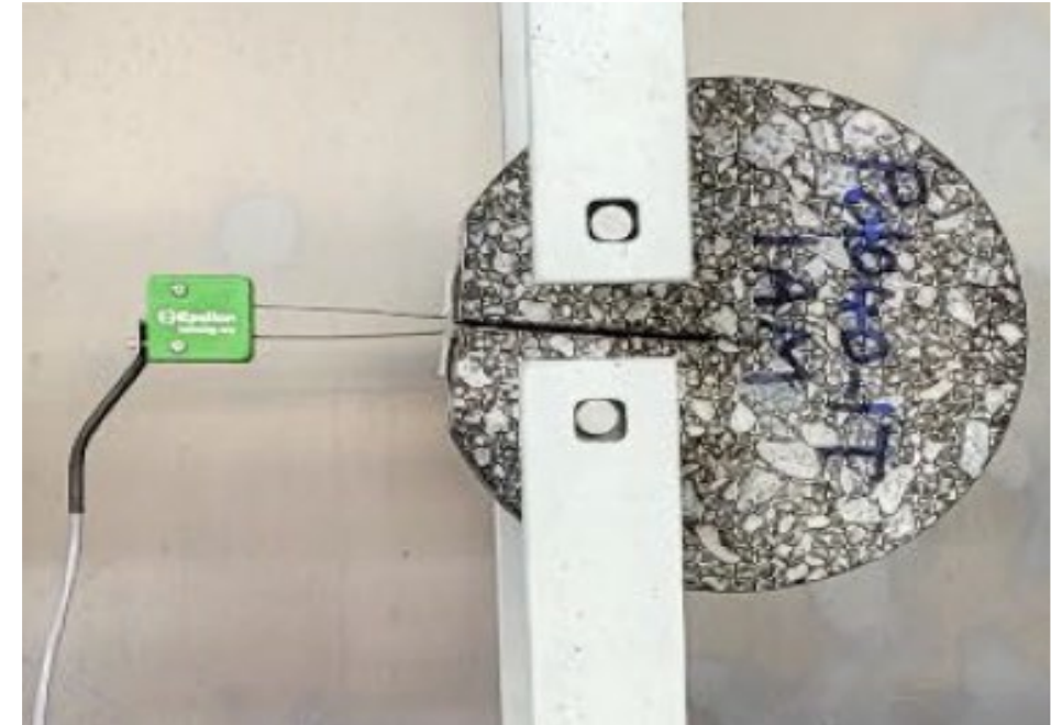
DISCK-SHAPED COMPACT TENSION ASTM D7313-13
