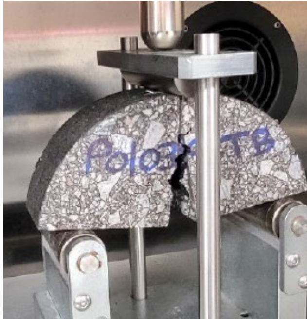
SCB CRACKING RESISTANCE (I-FIT) AASHTO T 393
