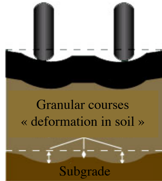
Rutting by deformation of granular layers
