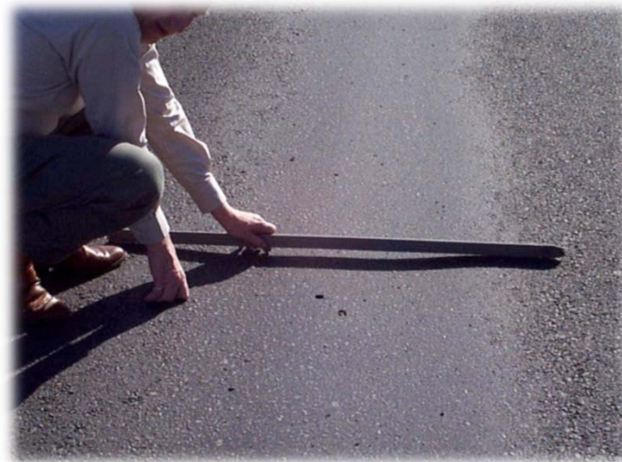
PG 67-22 unmodified, 15mm rut
