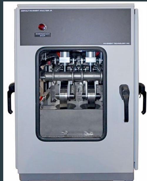
Asphalt Pavement Analyzer Testing – Rutting AASHTO T340
