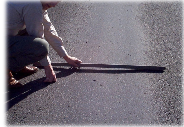
PG 67-22 unmodified, 15mm rut
