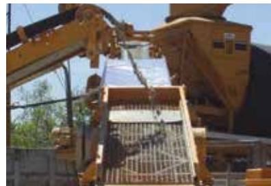
Aggregate delivery from the cold bins to the drum. Increased height may cause segregation.
